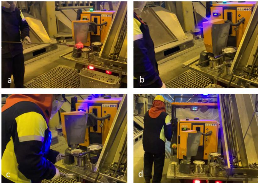
Figure 3. Chemical analysis of liquid aluminum from reduction cells.
